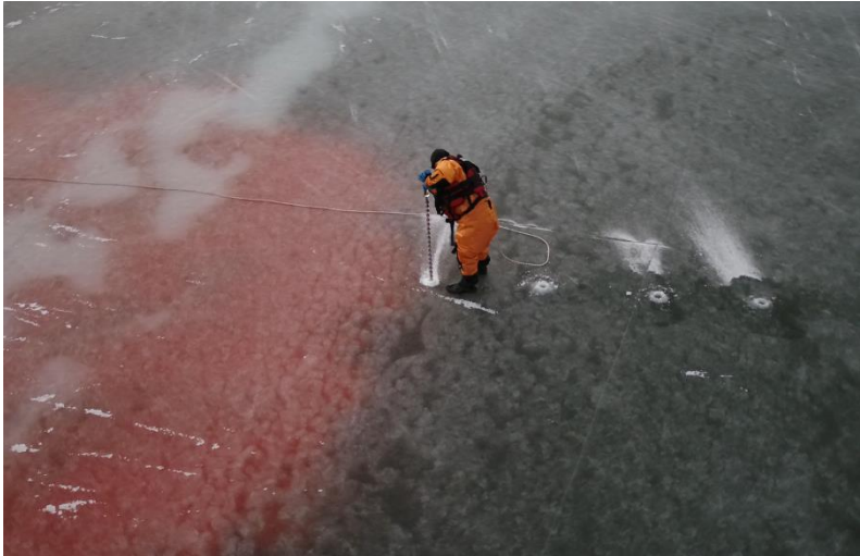
Delineation under ice using approved dye as oil surrogate.
