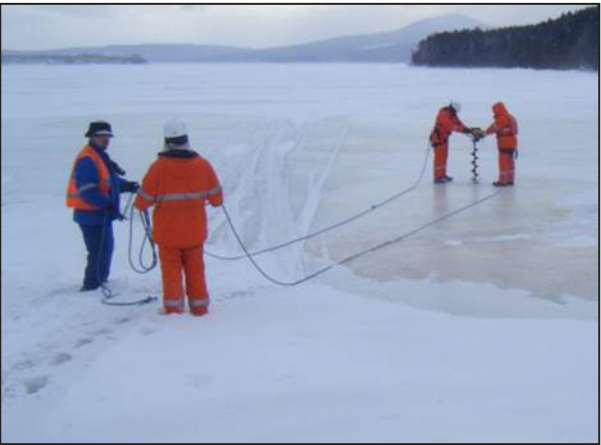
Ice profiling teams with body harnesses and safety lines to check for ice thickness and conditions.
