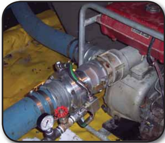
4" Trash Pump w/Annular Injection Flange
