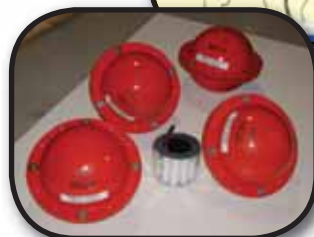
Orion Spill Tracking System w/40 Buoys
